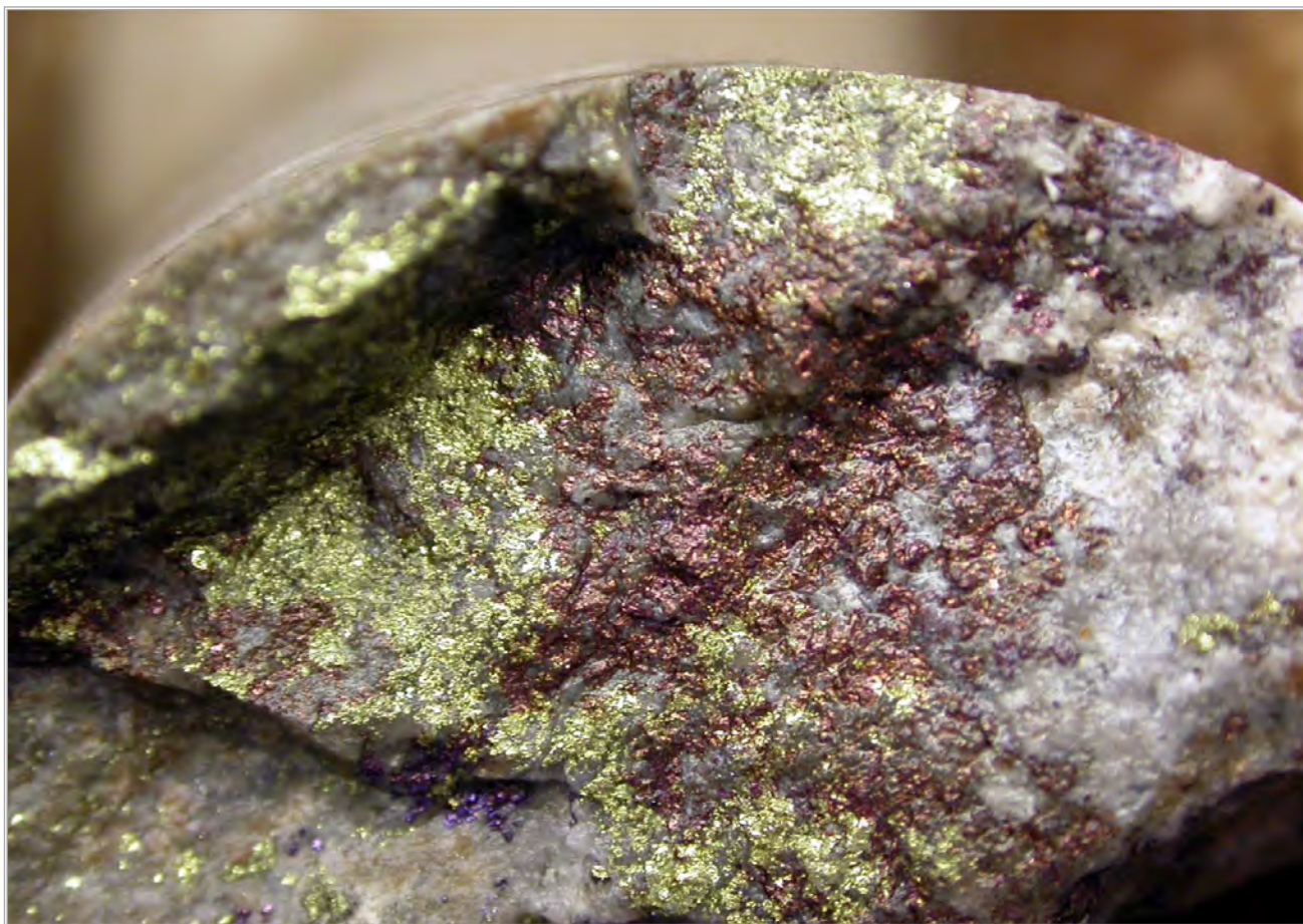
Figure 7-9: Drill Core Photograph Showing Chalcopyrite and Bornite Mineralization
