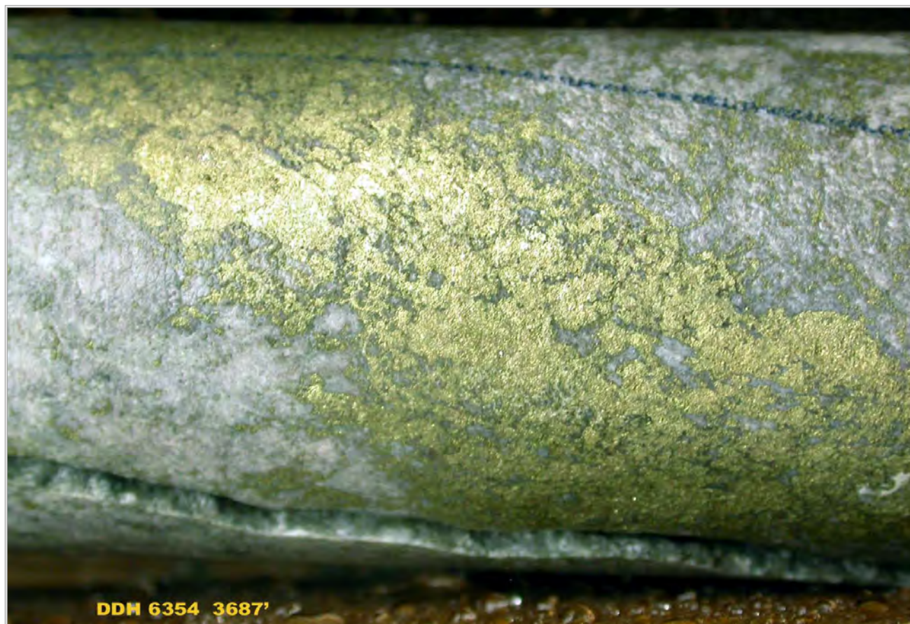
Figure 7-8: Drill Core Photograph Showing Chalcopyrite Mineralization
