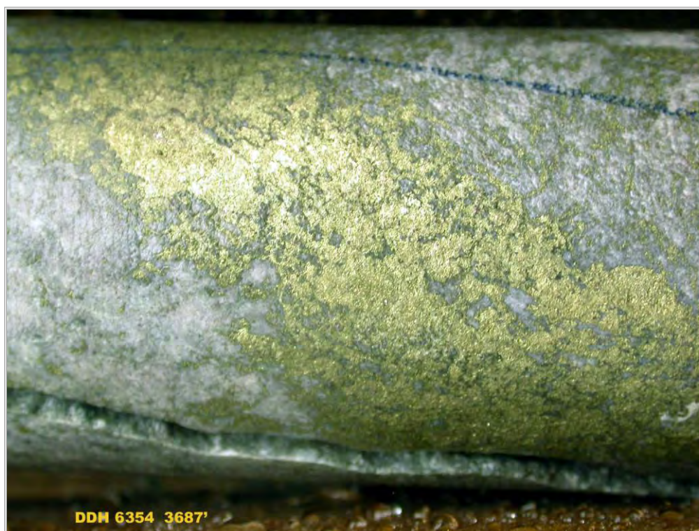
Figure 7.5.1 Drill Core Photograph Showing Chalcopyrite Mineralization
